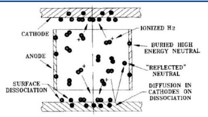
Sputtering Ion Pumps pump hydrogen gas differently. Hydrogen pumping is a two-step process:
