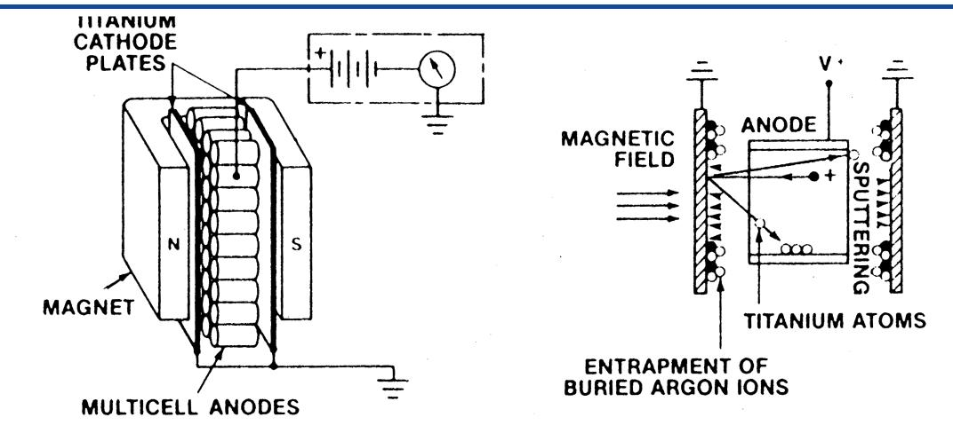
In a diode ion pump, both cathode plates are commonly made of titanium, due to its high sputtering yields and chemical reactivity
