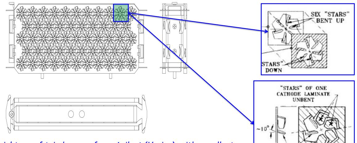
A special type of triode pump from Agilent (Varian), with excellent noble gas pumping, and improved long-term performance over stripstyle triode pump.
