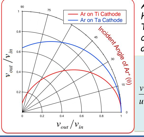
Argon neutrals clearly maintain much higher kinetic energy upon striking a Ta cathode as compared to a Ti cathode, specially at large incident angles.
